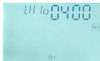
▶ Repress “SET” button, temperature “40°C” blinks on screen
