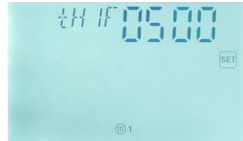
▶ Press button “+”, “tH 1F 05:00” displays on screen, the switch-off time and temperature for the first schedule of heating function can be set.
