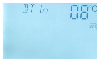
▶ Press “+/-” button, to adjust the value of switch-on DT, adjustable range (OFF+2 °C) ~ 20 °C, factory setting is 8 °C
