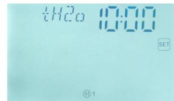
▶ Press button “+”, “tH 2F 10:00” displays on screen, the switch-off time and temperature for the second schedule of heating function can be set.
