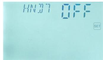
**Note:** when manual mode is activated,
