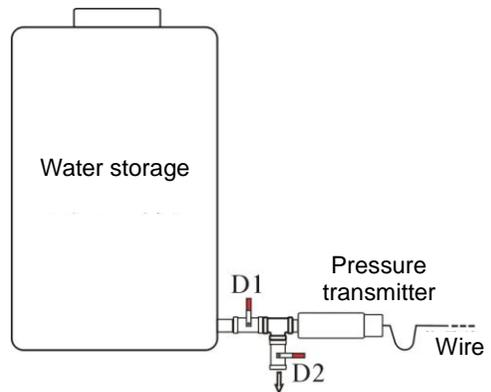
**Mounting the pressure water level transmitter**
